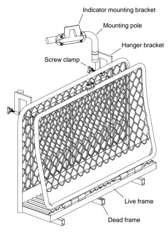
*Note:* The sheep crate can also be used on the ground on a firm level surface. However, due to its lightweight construction, it needs to be restrained to prevent it sliding about as animals enter and exit.
